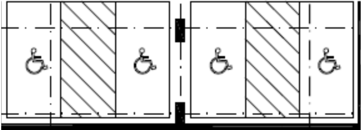
Figure 21: 'Shared zone' spaces (shown marked with a diagonal line) located between accessible parking spaces
